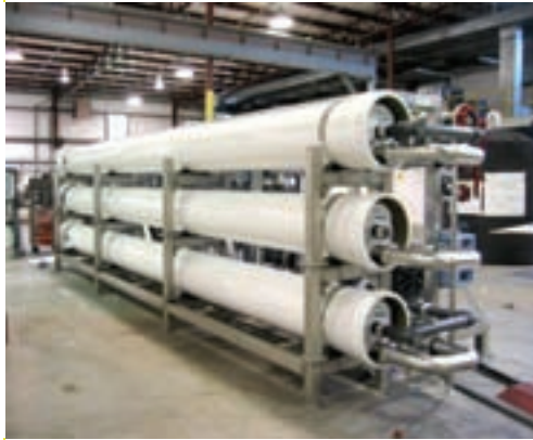
These reverse osmosis vessels are the largest of their kind, capable of treating more than 500,000 gallons per day.
